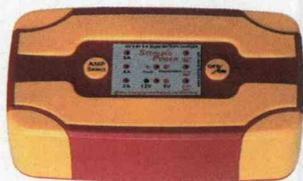
The new unit will charge 6V or 12V batteries, with six battery types: flooded, gel, AGM, advanced AGM, calcium and lithium. It has three basic stages – bulk, absorption and float – but if it detects the initial voltage is between 7.5V and 10.5V, it goes into pulse mode to rescue a dead battery. You can also choose a 15.5V desulphation mode at any time. The maximum current can be set to 3A, 5A or 7A.
