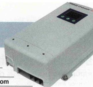
Merlin did not have a portable unit available at the time of test, so they sent us their smallest fixed unit, the Kisae 20A. This is another sophisticated charger, with a corresponding price tag. It has three outputs, one for the main service bank and two more for engine start and generator start batteries. In use, the main bank gets the priority charging until it has reached float stage, when charging moves to the other two.
