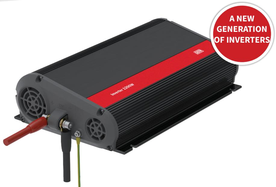
Integrated transfer switch automatically ensures that 230V power is supplied from a connected mains outlet when possible. This prevents the inverter from drawing power from the battery, allowing it to recharge. When mains power is disconnected power supply is switched back to the inverter.
